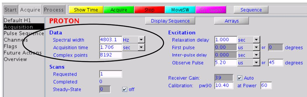
The simplest way to set the Spectral Width is to type the ppm range that you want into the boxes on the “Acquire >Default H1 Page”. This will set the center of the spectrum (tof) to the middle of the desired ppm range.
