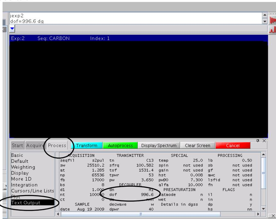
To determine the number of scans for your available time, type `time(hours,minutes)`. For example, if I have 1 hour and 15 minutes, type `time(1,15) dg`. This will set the number of scans (nt) to the appropriate number. Type `bs=16 ga wbs('wft')` in the command window. This will start the experiment and show you the carbon experiment at the completion of every 16 scans.
