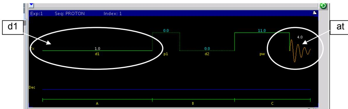
To change d1 or at, type `d1=#` and `at=#` on the command line. Type `dg` to refresh the parameter list and `dps` to refresh the pulse sequence.
