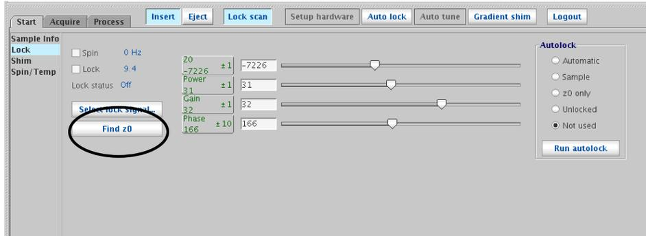
Click the “Lock Scan”, uncheck the “Lock Box” to turn off the lock. Adjust (raise or lower as necessary) the Power and Gain until the signal completely appears on the screen.
