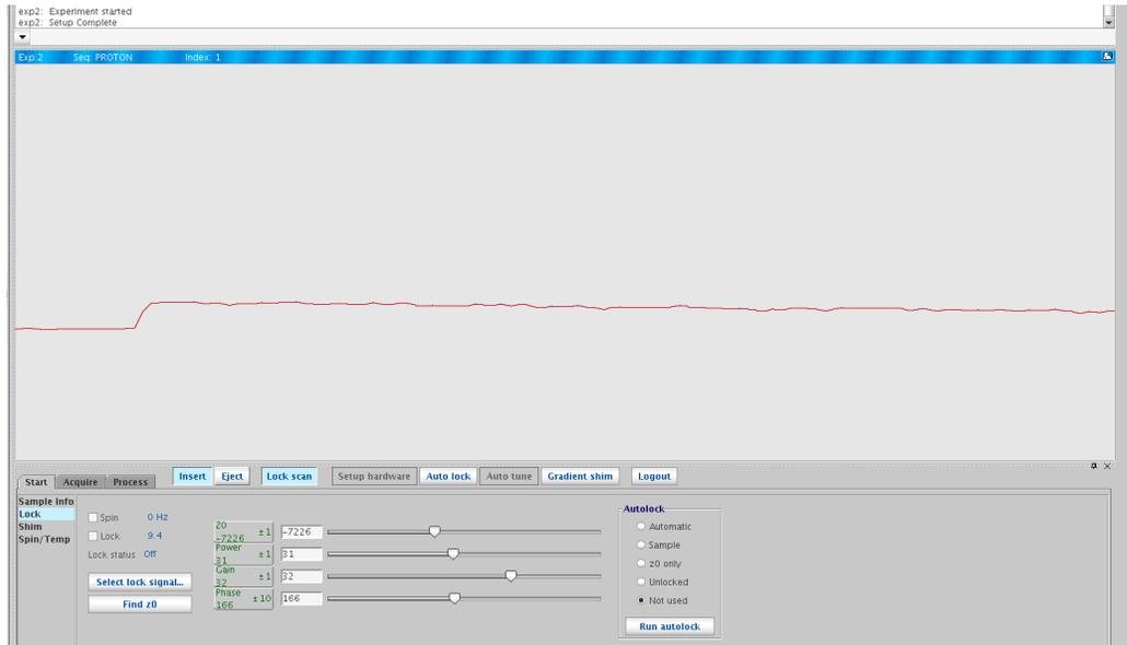
Adjust Z0 to maximize the lock signal. For best results adjust Z0 until signal is maximized, then adjust phase until the signal is maximized. Clicking the middle wheel of the mouse will change the steps of Z0, power, gain and phase to 1, 10 or 100. If the lock level is fluctuating at a low power level, then lower the gain.
