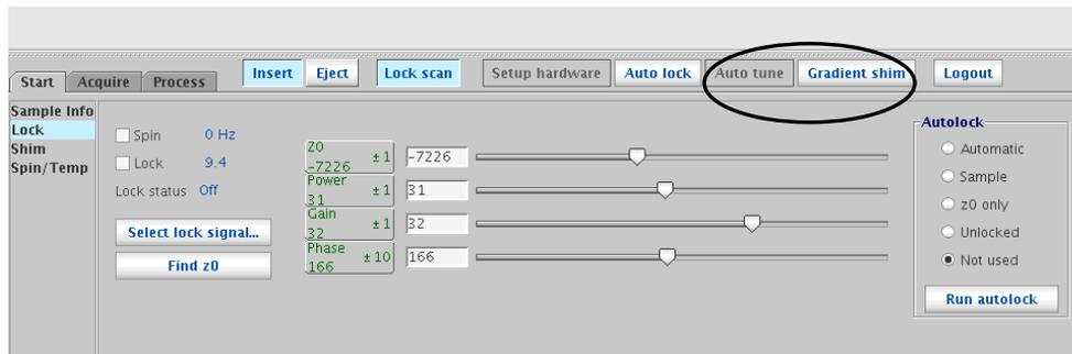
Alternatively, you may manually shim using the buttons on the “Shim Page” of the “Start Tab” to maximize the lock signal.
