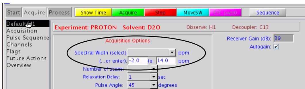
Alternately, the cursors and the movesw command can be used: Place the cursors around the peaks and type movesw. This will automatically change the sw to the position of the cursors and adjust tof to the halfway point between the cursors.
