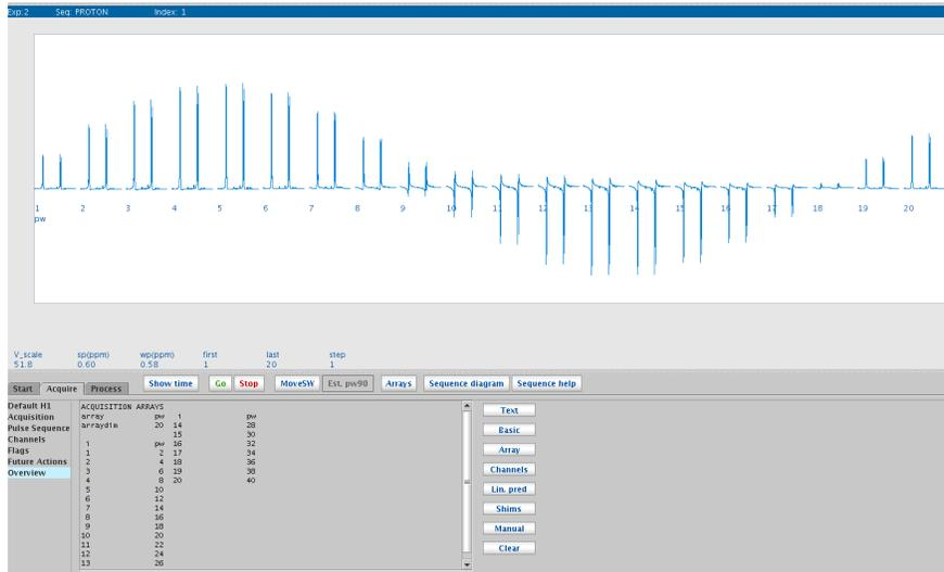
The  $90^\circ$  pw is calculated by taking the  $360^\circ$  pw and dividing it by 4. The  $360^\circ$  pw is identified as the second null point in the curve. In this example, the 18<sup>th</sup> spectra is around the  $360^\circ$  pw. This corresponds to 36  $\mu$ s.
