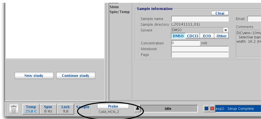
Click on the down arrow to view the probe file options. Select the desired file and close the box. For the Chempack training, use the Cold\_HCN\_2 probe file.
